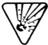
Figure 5. Explosion symbol (Used with permission of WorkSafeBC)
