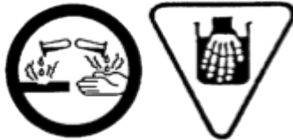
Figure 11. Corrosive material symbol (Used with permission of WorkSafeBC)
