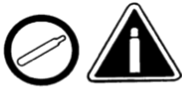
Figure 4. Compressed gas symbol (Used with permission of WorkSafeBC)
