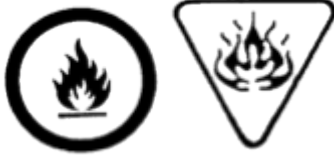
Figure 6. Flammable and combustible material symbol (Used with permission of WorkSafeBC)
