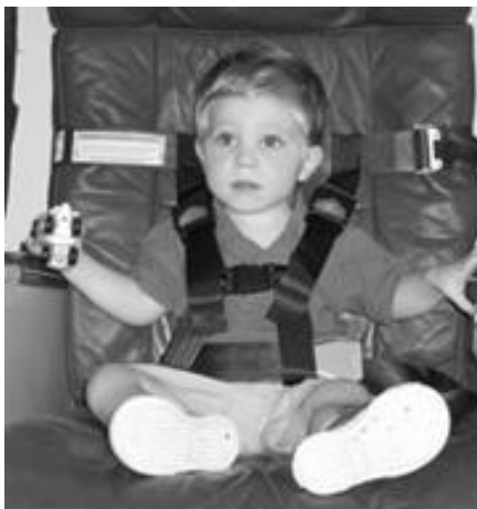
CSD – Child Safety Device – Fastening Children System device USA approved for aircraft use only. Recommended for children between 10 and 20 Kg
