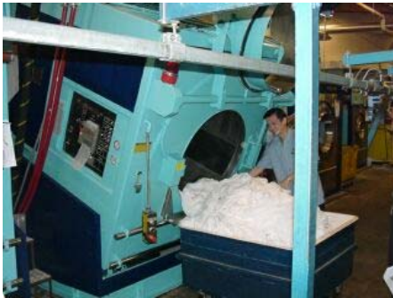
Mechanical tilting of the washing machine reduces stretching and force to retrieve laundry
