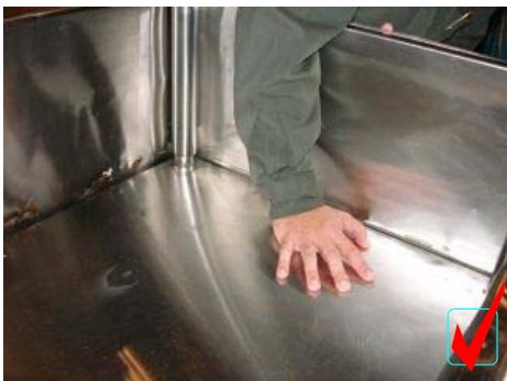
Using bins with self-elevating base to reduce bending of the back when retrieving laundry
