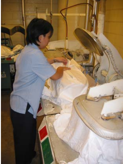
Laundry operators are exposed to heat from hot presses
