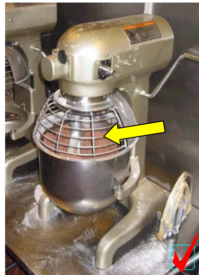
Example of machine guarding in the kitchen
