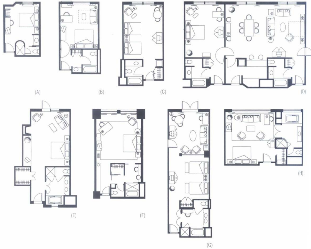
Typical and unique guestroom layouts Guestroom plans. (A) Economy queen room, 220 ft 2 (20.5 m 2 ) saves space with sink/vanity outside bathroom and one bed. (B) Mid-scale king room, 320 ft 2 (30 m 2 ) shows how placing the bed against the bathroom wall increases useable space. (C) First-class double-double room, 365 ft 2 (34 m 2 ) with typical furnishings. (D) Three-bay conference suite, 1,160 ft 2 (108 m 2 ) combines a two-bay public area with wall-bed, lounge seating, work area, full bathroom, and wet bar with a typical guestroom, and second connecting room. (E) Luxury resort room 550 ft 2 (51 m 2 ) introduces five-fixture bathroom and fireplace (Four Seasons, Scottsdale). (F) International luxury guestroom, 530 ft 2 (49 m 2 ) features carefully detailed built-in storage, sliding doors, and glass partitions for an open effect (Park Hyatt, Hamburg). (G) Luxury casino-hotel room, 665 ft 2 (62 m 2 ) features large bathroom, queen-queen beds, and separate living area (The Venetian, Las Vegas). (H) Rotated room configuration, 530 ft 2 (49 m 2 ) places whirlpool tub on the exterior wall of spacious bathroom and features unusually wide guestroom space (The Ritz-Carlton Millenia, Singapore). (For vacation ownership, all-suite, and extended-stay units see Chapters 4 and 8.)
